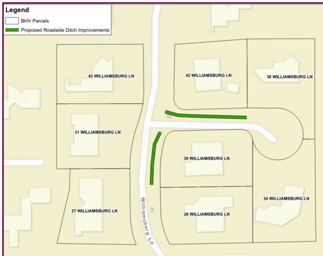
Figure 1. Proposed Roadside Ditch Improvements
