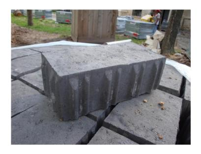
PERMEABLE PAVERS MIN. 3 1/8" (80mm) THICK
